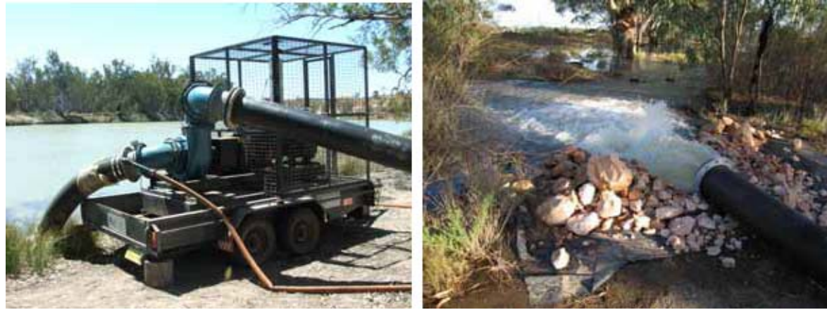
Pump set-up on Murray River for watering wetlands in the Lower Murray-Darling.
